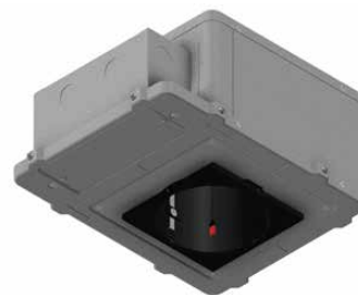
FRM2-4W-S-CP HOUSING for FLANGELESS INSTALLATION with FLS-4 SQUARE FLAT trim in Wood/Stone ceilings. CCEA plenum rated for City of Chicago environmental air spaces and rated for direct contact with spray-foam insulation.
