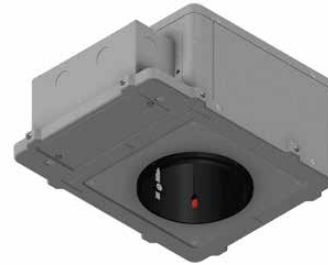
FRM2-4W-R-CP HOUSING for FLANGELESS MOUNTING ROUND FLAT trim in Wood/Stone ceilings. CCEA plenum rated for City of Chicago environmental air spaces and rated for direct contact with spray-foam insulation.
