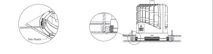
5e. Re-install temporary dust cover until after ceiling has been completely finished.
