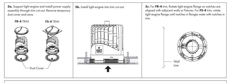
**5d.** Locate (4) four locking screws. While applying upward pressure on light engine flange, hand tighten using supplied 3/32" hex-key. Ensure light engine flange is tight against trim and aligned with trim notches.
