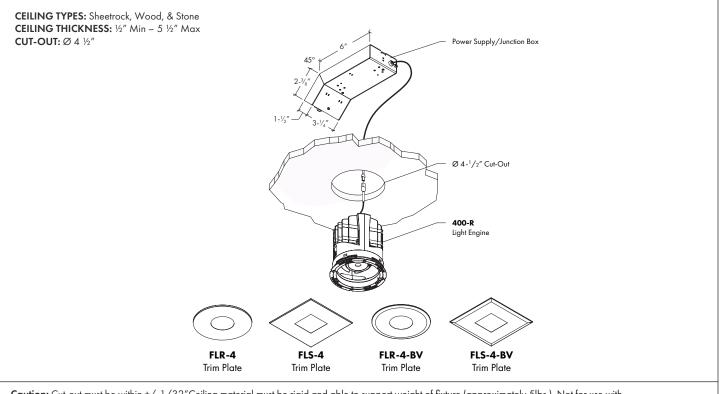
**Caution:** Cut-out must be within +/-1/32" Ceiling material must be rigid and able to support weight of fixture (approximately 5lbs.). Not for use with acoustic tile or non-rigid ceiling materials.
