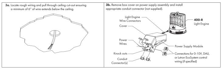
3c. Review wiring diagrams on page 10 & 11, wire accordingly. Place all wiring and connectors back in power supply box and replace cover.
