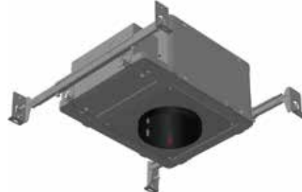
FRM2-4T-CP MOUNTING FRAME for FLANGED INSTALLATION with FLR-4/FLR-4-BV Round or FLS-4/FLS-4-BV SQUARE trims in Acoustic Tile/Fabric ceilings. CCEA plenum rated for City of Chicago environmental air spaces and rated for direct contact with spray-foam insulation.
