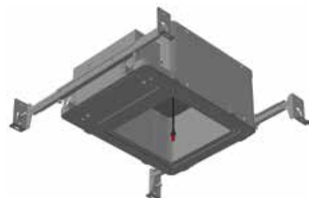
FRM2-S6-CP MOUNTING FRAME for FLANGELESS INSTALLATION with FS-4 SQUARE trim in sheetrock ceilings. CCEA plenum rated for City of Chicago environmental air spaces and rated for direct contact with spray-foam insulation.
