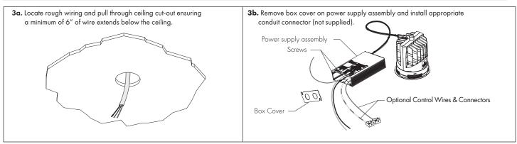
3c. Review wiring diagrams on page 10 & 11, wire accordingly. Place all wiring and connectors back in power supply box and replace cover.
