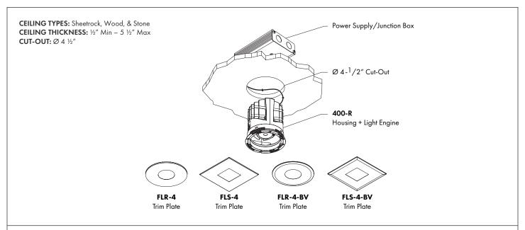
Caution: Cut-out must be within +/-1/32"Ceiling material must be rigid and able to support weight of fixture (approximately 5lbs.). Not for use with acoustic tile or non-rigid ceiling materials.
