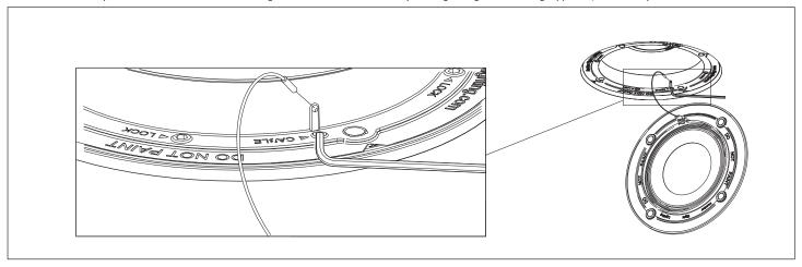
2c. Align trim plate with magnets and install.
