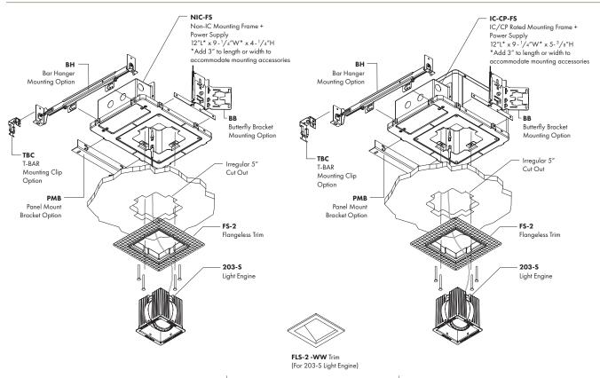
CEILING TYPES: Sheetrock | CEILING THICKNESS: 1/2" Min to 1-1/2" Max | CUT-OUT: 5" Irregular
