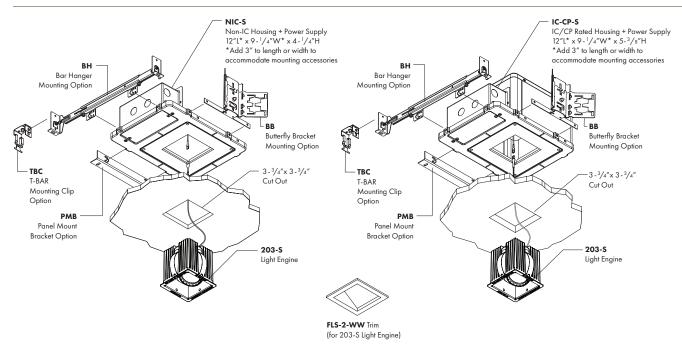
CEILING TYPES: Sheetrock, Wood, Stone & Acoustic Tile | CEILING THICKNESS: 1/2" Min to 1-1/2" Max | CUT-OUT: 3-3/4" x 3-3/4" x 3-3/4"
