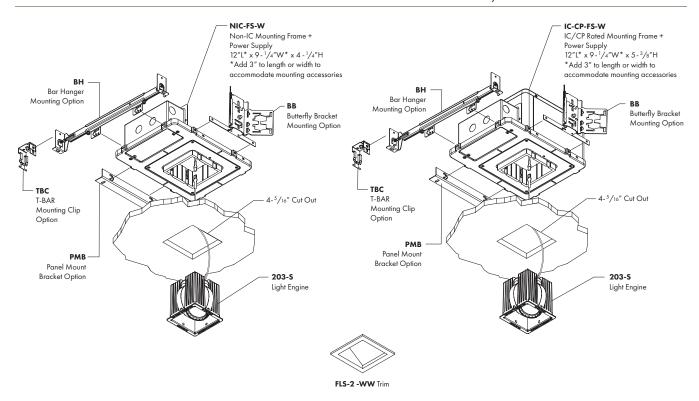
CEILING TYPES: Wood/Stone CEILING THICKNESS: 1/2" Min to 1-1/2" Max CUT-OUT: CUT-OUT: 4-5/16" x 4-5/16"
