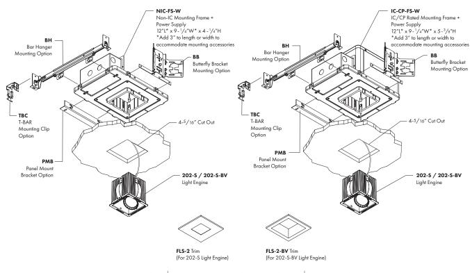
**CEILING TYPES:** Wood/Stone | **CEILING THICKNESS:** 1/2" Min to 1-1/2" Max | **CUT-OUT:** 4 - 5/16" x 4 - 5/16"
