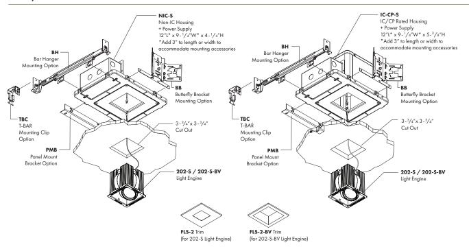
CEILING TYPES: Sheetrock, Wood, Stone & Acoustic Tile | CEILING THICKNESS: 1/2" Min to 1-1/2" Max | CUT-OUT: 3-3/4" x 3-3/4"
