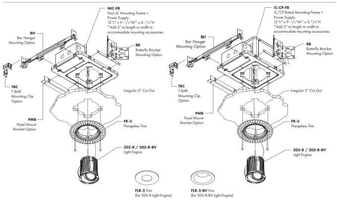
CEILING TYPES: Sheetrock | CEILING THICKNESS: 1/2" Min to 1-1/2" Max | CUT-OUT: 5" Irregular
