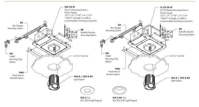
CEILING TYPES: Wood/Stone CEILING THICKNESS: 1/2" Min to 1-1/2" Max CUT-OUT: Ø 4-5/16"
