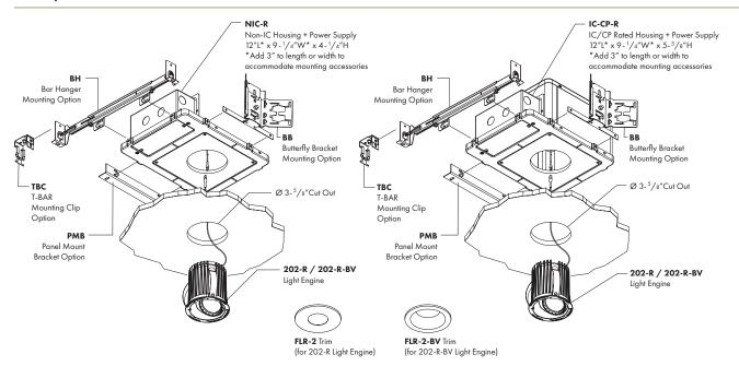
CEILING TYPES: Sheetrock, Wood, Stone & Acoustic Tile | CEILING THICKNESS: 1/2" Min to 1-1/2" Max | CUT-OUT: Ø 3-3/4"
