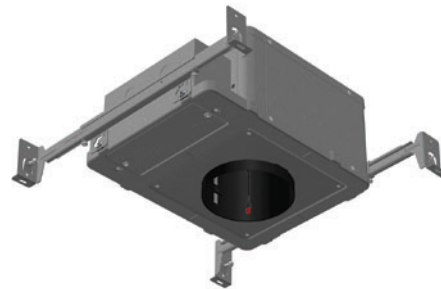
FRM2-4T-CP MOUNTING FRAME for FLANGED INSTALLATION with FLR-4/FLR-4-BV Round or FLS-4/FLS-4-BV SQUARE trims in Acoustic Tile/Fabric ceilings. CCEA plenum rated for City of Chicago environmental air spaces and rated for direct contact with spray-foam insulation.
