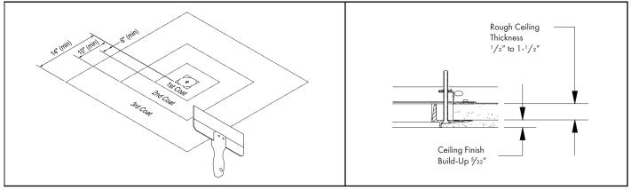
**4f.** First Coat - Apply USG "Durabond" setting-type joint compound for embedding the perforated flange and fiberglass mesh tape following the manufacturer's instructions and warnings for outside corners and trim. The compound should extend a minimum of 6" from the trim edge. Allow first coat to dry completely and remove any high spots by lightly sanding before applying the second coat.
