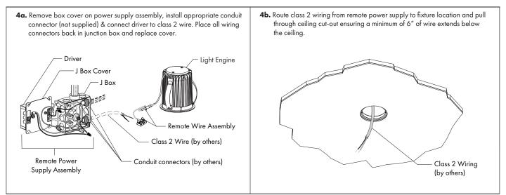
**STEP 5** – LIGHT ENGINE WIRING AND INSTALLATION
