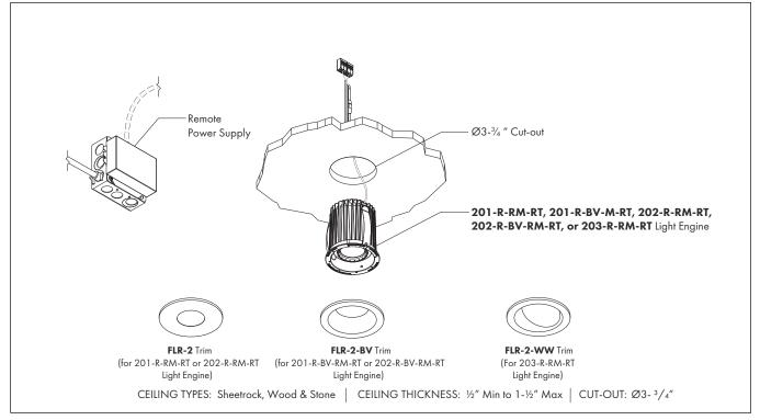
**Caution:** Cut-out must be within  $\pm \frac{1}{32}$ " Ceiling material must be rigid and able to support weight of fixture (approximately 5lbs.). Not for use with acoustic tile or non-rigid ceiling materials. Minimum of  $4-\frac{1}{2}$ " rough ceiling space required for installation.
