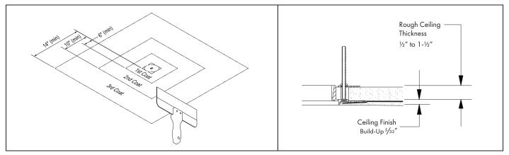
**3f.** First Coat - Apply USG "Durabond" setting-type joint compound for embedding the perforated flange and fiberglass mesh tape following the manufacturer's instructions and warnings for outside corners and trim. The compound should extend a minimum of 6" from the trim edge. Allow first coat to dry completely and remove any high spots by lightly sanding before applying the second coat.
