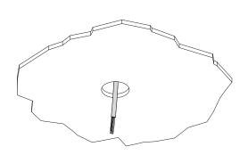
**3b.** Remove box cover on power supply assembly and install appropriate conduit connector (not supplied).
