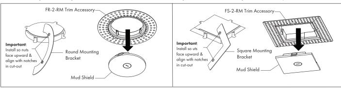
3b. Rotate trim to be aligned with adjacent walls or fixtures as shown below. Note: hand tighten trim screws. A power driver is not recommended.
