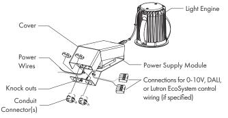
3c. Review wiring instructions on page 9 & 10, wire fixture accordingly. Place all wiring connectors back in power supply box and replace cover.
