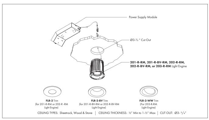
**Caution:** Cut-out must be within  $\pm \frac{1}{32}$ " Ceiling material must be rigid and able to support weight of fixture (approximately 5lbs.). Not for use with Acoustic tile or non-rigid ceiling materials. Minimum of 5-1/2" rough ceiling space required for power supply installation.
