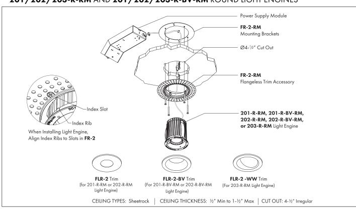
CAUTION: For use with sheet rock material only. Cut-out must be within ± 1/16". Minimum of 5-1/2" rough ceiling space required for power supply module installation.
