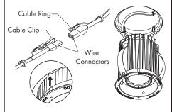
Align Index Ribs & Slots when installing Light Engine.
